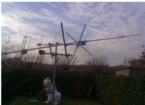
2x 14 elements 4 wl yagi antenna
